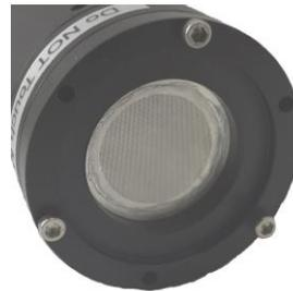
4. Install the Copper Shield, P/N 2410-508 or .2400-508
