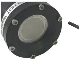
2. Install O-ring from sloped faceplate into the inset faceplate.
