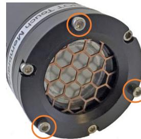
**CAUTION:** It is important to ensure the copper screen does not contact the stainless steel head cap screws or the sensor membrane as this will result in galvanic corrosion of the head screws. If the Pumped Head Assembly is used the copper screen can be used but you must install longer screw
