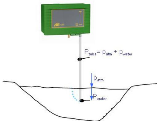
Figure 3: Determination of water level
