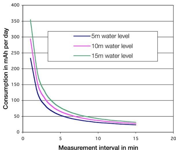
Diagram 3: Power consumption with minimal water level changes
