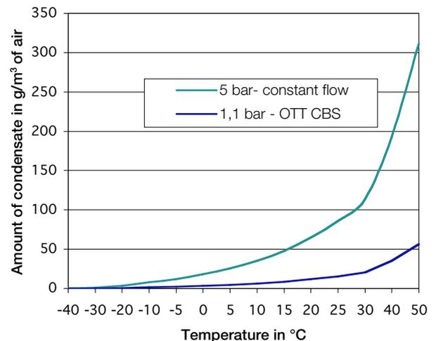
Diagram 2: Condensate at 80 % relative humidity per m<sup>3</sup>
