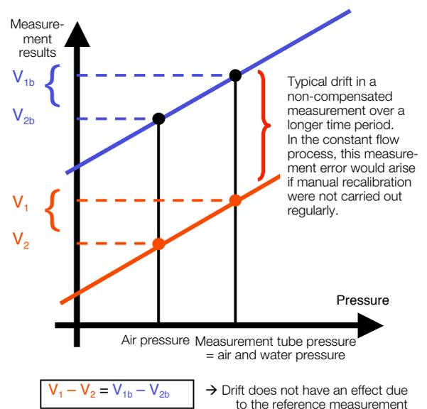
Figure 4: OTT CBS Drift-free Measurement Principle
