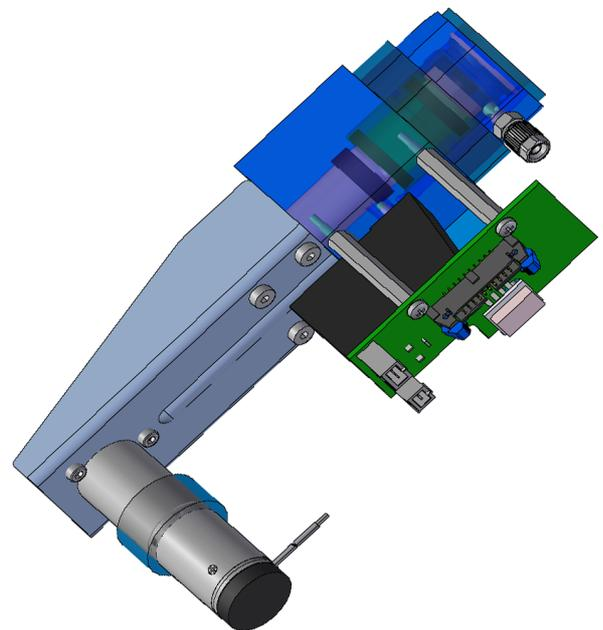
Figure 2: Motor-gear-pump Unit + Pressure Measurement Unit
