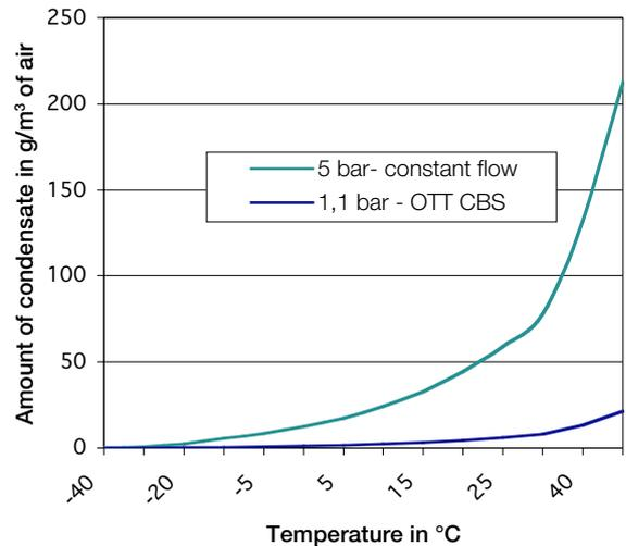
Diagram 1: Condensate at 60 % relative humidity per m<sup>3</sup>
