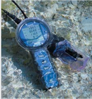
The Quanta Field Display – waterproof (IP 67/NEMA 6), robust, compact, easy to use, simple menu-driven operation
