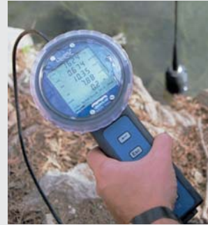
The Quanta Field Display – displays readings of up to 5 parameters simultaneously
