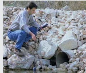
Portable online-measurement of water quality at a waste-water outlet
