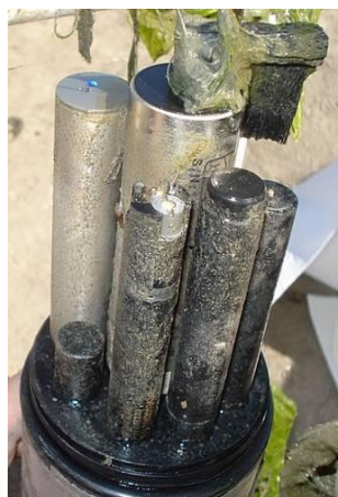
Above: sensors fouled after deployment (l) vs. sensors deployed with copper tape (r)
