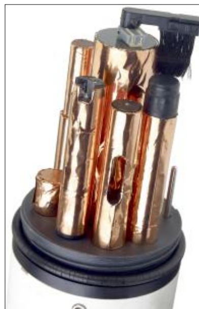
Above: sensors wrapped with copper tape
