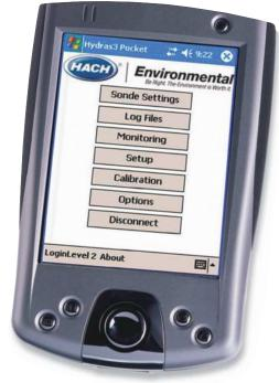
Hydras 3 Pocket includes complete capability to set-up, edit, and download log files.
