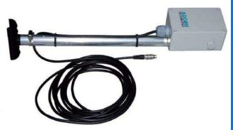
Its extremely low power consumption and robust poly-carbonate housing, make the device ideally suited for permanent outdoor operation. A Goretex breather vent provides pressure compensation; the aluminium arm allows mounting on Adcon's standard aluminium poles; and a 4m cable with Adcon's standard 7-pin connector makes the device compatible with most Adcon RTUs (A723, A733, A753 and A755).
