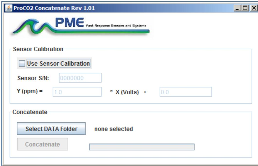
ProOCO2Concatenate reads and concatenates the files recorded by the ProOCO2 Logger. Software produces CAT.txt in the same folder as selected for the data. CAT.txt contains all the original measurements and contains two additional statements of time. If the Use Sensor Calibration is checked the CAT file will contain an additional column of CO2.
