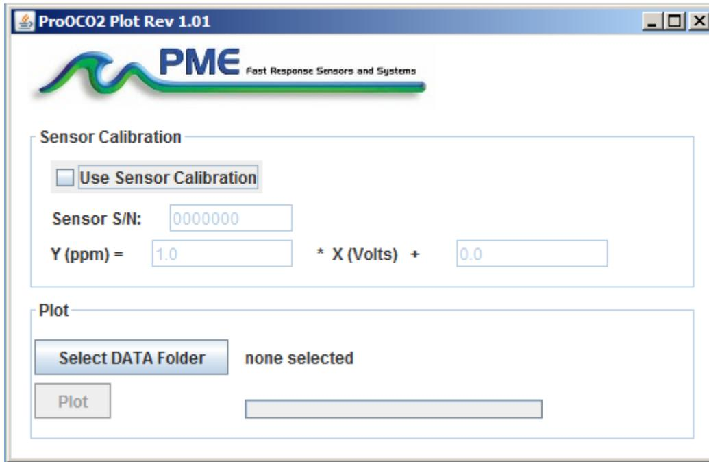
ProOCO2Plot plots the files recorded by the ProOCO2 Logger. The software reads all ProOCO2 files in a folder, except the CAT.txt file. The software will also compute CO2 saturation from the voltage measured of the sensor. To do this software must be given the sensor calibration. The sensor manufacturer supplies the sensor calibration. If the Use Sensor Calibration is checked the plot will display calibrated values. If not checked the plot will display sensor output in Volts.
