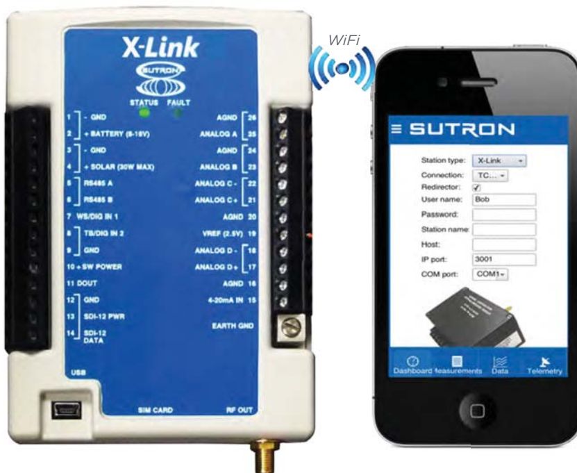
Little Box. Big Data. X-Link dimensions are 3.8" x 5.3" x 1.3" (96.5mm x 134.6mm x 33.0mm - approximately the size of an iPhone).
