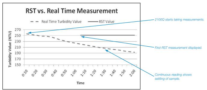
Although the sample continuously settles out of solution, the RST calculated value does not change.
