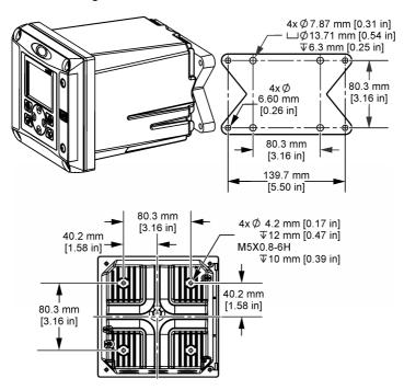
Figure 4 Panel mounting dimensions
