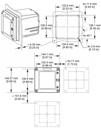
Note: If using the bracket (optional) for panel mounting, push the controller through the hole in the panel and then slide the bracket over the controller on the back side of the panel. Use the four 15 mm pan head screws (supplied) to attach the bracket to the controller and secure the controller to the panel.
