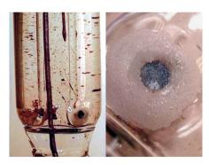
eramic diaphragm by a sulphide deposit
