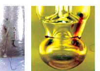
Correctly functioning ceramic diaphragm, effluence of electrolytes (red liquid)
