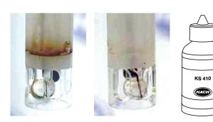
Contaminated (left) and clean (right) gel electrolyte
