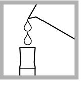
2. Prepare the blank: Fill a 25-mL mixing cylinder to the 25-mL mark with deionized water.
