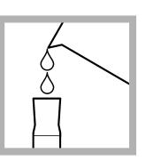
**3. Prepare the sample:** Fill a second 25-mL mixing cylinder to the 25-mL mark with sample.
