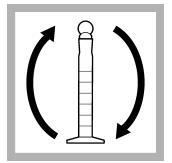
**5.** Close the two cylinders. Invert both cylinders several times to mix.
