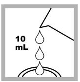
**8.** Pour 10 mL of each solution into two sample cells.
