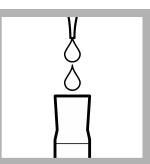
**6.** Add 5.0 mL of Sodium Carbonate Solution into each cylinder.
