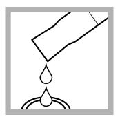
**24.** Prepare the sample: Pour the reacted arsenic absorber sample into a sample cell. Put the stopper on the sample cell.
