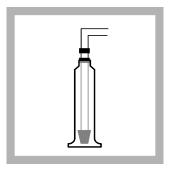
**18.** When the timer expires, set the heater power to off. Remove the cylinder/gas bubbler assembly as a unit.
