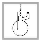
**10.** Use a serological pipet to add 1 mL of Stannous Chloride Solution to the distillation flask.
