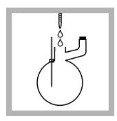
**11.** Use a serological pipet to add 3 mL of Potassium lodide Solution to the distillation flask. Put the cap on the flask.
