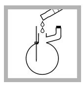
**9.** Use a graduated cylinder to add 25 mL of Hydrochloric Acid ACS to the distillation flask.
