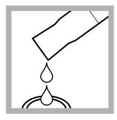
**20. Prepare the blank:** Fill a dry 10-mL sample cell with unreacted arsenic absorber solution. Put the stopper on the sample cell.
