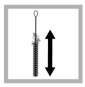
**13.** Clean the sample cell immediately after each test with soap, water and a brush.
