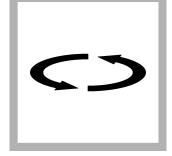
4. Swirl to mix. The sample becomes cloudy if barium is in the sample. If the powder does not dissolve well, mix the sample and reagent in a 25-mL mixing cylinder, then pour into the sample cell.
