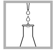
**5. Prepare the blank:** Use a pipet to add 2.0 mL of deionized water into a 125-mL Erlenmeyer flask.
