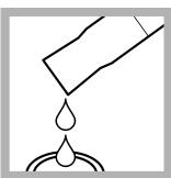
**10.** When the timer expires, pour at least 10 mL from each flask into separate sample cells.
