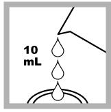
2. Prepare the blank: Fill a sample cell with 10 mL of deionized water.
