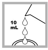
2. Prepare the blank: Fill the sample cell with 10 mL of deionized water.
