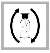
**7.** Quickly invert the AccuVac Ampul several times to mix.
