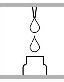
6. Prepare the sample: Remove the cap from a Free Chlorine DPD Test 'N Tube. Fill the vial to the top of the label with sample.
