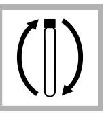
7. Put the cap on the vial. Invert slowly for 20 seconds to dissolve the powder.
