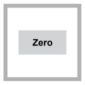
**3.** When the flow stops, push **ZERO**. The display shows 0.00 mg/L CL<sub>2</sub>.
