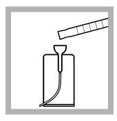
9. Fill the funnel of the Pour-Thru Cell with the reacted sample from the mixing cylinder. It is not necessary to pour all of the sample into the Pour-Thru Cell; approximately half of the sample can be discarded.
