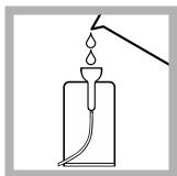
**2.** Pour 50 mL of sample into the Pour-Thru Cell.
