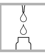
6. Prepare the sample: Remove the cap from a Total Chlorine DPD Test 'N Tube. Fill the vial to the top of the label with sample.
