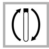
7. Put the cap on the vial. Invert slowly for 20 seconds to dissolve the powder.
