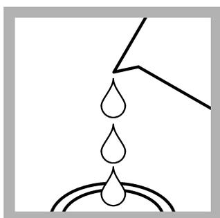
**2. Prepare the blank:** Fill a sample cell to the 5-mL mark with sample.
