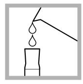
**10. Prepared Sample:** Be careful to prevent agitation and slowly fill the cylinder to the 50-mL mark with sample.
