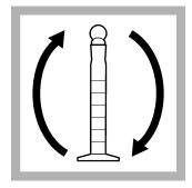
**11.** Put the stopper on the mixing cylinder. Invert the mixing cylinder carefully twice to mix.
