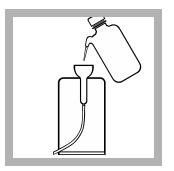
**19.** Flush the Pour-Thru Cell with at least 50-mL of deionized water immediately after use.
