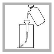
**15.** Flush the Pour-Thru Cell with at least 50-mL of deionized water immediately after use.
