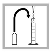
**8.** Use a TenSette Pipet with a clean tip to add 1 mL of indicator from the ampule to the same mixing cylinder.
