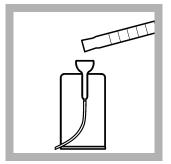
**16.** When the timer expires, pour the contents of the mixing cylinder into the Pour-Thru Cell.
