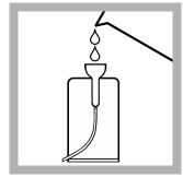
**2.** Pour 50 mL of sample into the Pour-Thru Cell.
