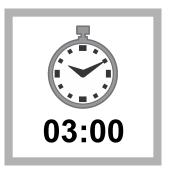
**12.** Start the instrument timer. A 3-minute reaction time starts. Monitor the time and measure the reacted sample 3-4 minutes after mixing the sample and reagents.
