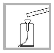
**13.** When the timer expires, pour the contents of the mixing cylinder into the Pour-Thru Cell.
