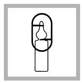
**7.** Open one ampule of DPD Indicator Solution for Ultra Low Range Chlorine.
