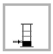
**13.** Push the valve button on the OriFlo barrel assembly in ("closed" position). Put the barrel assembly into its stand.
