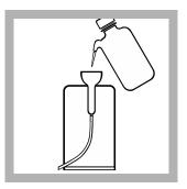
**24.** Flush the Pour-Thru Cell with at least 50-mL of deionized water immediately after use.
