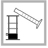
**20.** When the timer expires, pour the contents of the mixing cylinder into the barrel.
