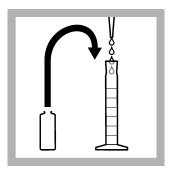
**8.** Use a TenSette Pipet with a clean tip to add 1 mL of indicator from the ampule to the same mixing cylinder.
