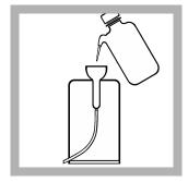
**2.** Flush the Pour-Thru Cell with at least 50-mL of deionized water.
