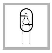
**5.** Open one ampule of ULR Chlorine Buffer Solution.
