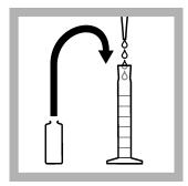
**6.** Use a TenSette Pipet with a clean tip to add 1 mL of buffer from the ampule to a clean and prepared 50-mL mixing cylinder.
