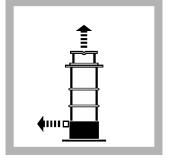
18. Pull the barrel valve button out to the "open" position. Pull the plunger up to separate it from the barrel assembly. Discard the remaining unfiltered sample. A new membrane may be necessary for very turbid samples. Alternatively, use a second Quick Filter unit with a new membrane filter installed.
