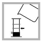
**14.** Pour approximately 50 mL of the original sample into the barrel. The lower ring on the barrel assembly shows about a 50-mL volume.
