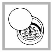
**4.** Install a new, 3-micron filter (white) into the cap recess. Wet the filter with drops of deionized water. Reassemble and hand-tighten the cap onto the plunger.
