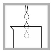
add 1.0 mL of Blanking Reagent to the beaker. Swirl to mix. The Blanking Reagent removes chlorine and chloramines from the water.
