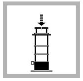
**15.** Insert the plunger into the barrel and slowly push the plunger down with even pressure until the plunger is fully seated.
