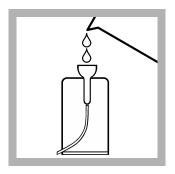
**14.** During the reaction period, flush the Pour-Thru Cell with the remaining dechlorinated water from step 4.
