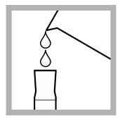
**10. Prepared Sample:**Prevent extra agitation while carefully filling the cylinder to the 50-mL mark with sample.
