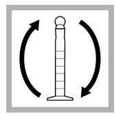
**11.** Put the stopper on the mixing cylinder. Carefully invert the mixing cylinder twice to mix.
