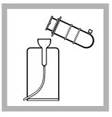
**16.** Pour the filtered, unreacted sample from the plunger reservoir into the Pour-Thru Cell.
