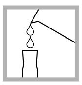
11. Fill the cylinder to the 50-mL mark with dechlorinated water from step 4. Keep the remaining dechlorinated water for step 14.
