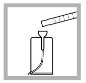
**16.** When the timer expires, pour the contents of the cylinder into the Pour-Thru Cell.
