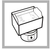
**5.** Keep the sample cell cap off. Put the prepared sample in a boiling water bath.
