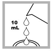
**15.** During the reaction, pour 10 mL from the mixing bottle into a sample cell for measurement. This is the **prepared sample**.
