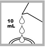
**10. Prepare the blank:** When the timer expires, fill a second sample cell with 10 mL of sample.
