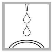
**9.** Remove the sample cell from the holder. Add 2 drops of CDTA Reagent for Ultra Low Range Hardness. Complete the remaining steps within 1–2 minutes.
