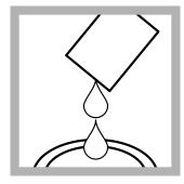
**4.** Add the contents of one Chlorophosphonazo Solution Pillow to the sample cell. A small quantity of solution that remains in the pillow does not affect results.
