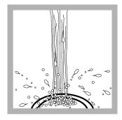
2. Clean a plastic sample cell and the cap three times with the test water. Make sure that the underside of the cap does not come in contact with surfaces that can contaminate it.
