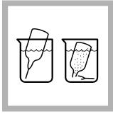
**3. Prepare the sample:** Collect at least 40 mL of sample in a 50-mL beaker. Fill the AccuVac Ampul with sample. Keep the tip immersed while the AccuVac Ampul fills completely.
