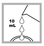
7. When the timer expires, pour 10 mL of the prepared sample from the mixing cylinder into the second sample cell.
