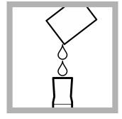
**4.** Add the contents of one FerroZine Iron Reagent Solution Pillow to the mixing cylinder.
