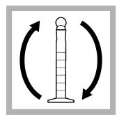
**5.** Put the stopper on the mixing cylinder. Invert the mixing cylinder several times to mix.
