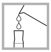
**3. Prepare the sample:** Fill a mixing cylinder to the 25-mL line with sample.
