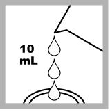
6. Prepare the blank: Fill a sample cell with 10 mL of deionized water.
