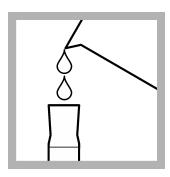
**5.** Fill a clean 25-mL mixing cylinder to the 25-mL mark with the prepared sample. Use the rest of the sample to prepare the blank.
