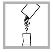
**3.** Add the contents of one FerroMo Iron Reagent 1 Powder Pillow to the mixing cylinder.
