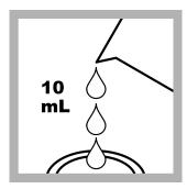
**6. Prepare the blank:** Fill a second sample cell with 10 mL of the prepared sample.
