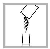
7. Develop the sample: Add the contents of one FerroMo Iron Reagent 2 Powder Pillow to the prepared sample in the 25-mL mixing cylinder.
