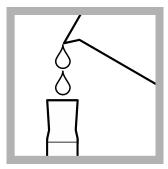
**2. Prepare the sample:** Fill a 50-mL mixing cylinder with 50 mL of sample.
