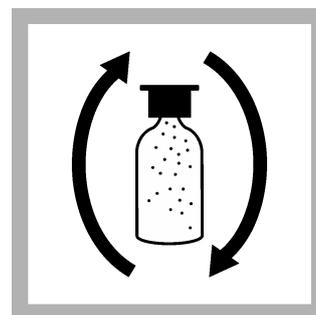
4. Quickly invert the AccuVac Ampul several times to mix. Undissolved powder will not affect accuracy.
