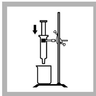
**11.** After the flow stops, fully compress the absorbent pad in the Extractor with the plunger. Safely discard the contents of the beaker. Slowly remove the plunger from the extractor. Make sure that the absorbent pad stays at the bottom of the Extractor when the plunger is removed. If the cotton plug moves up the column, push it back to the bottom with a clean, blunt rod.
