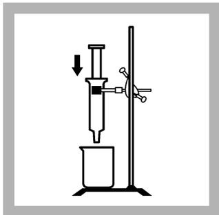
**13.** Let the Eluant Solution drip slowly from the extractor. When the flow stops, use the plunger to fully compress the absorbent pad.
