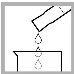
2. Fill a plastic graduated cylinder with 100 mL of the sample, then pour the measured sample into a clean 250-mL plastic beaker.
