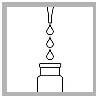
23. Remove the sample cell, then add 3 drops of pPb-6 Decolorizer Solution to the sample cell.
