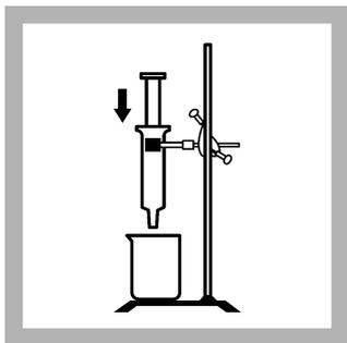
**9.** Soak the cotton plug in the extractor with deionized water, then compress it with the plunger. If the cotton plug moves up the column, push it back to the bottom with a clean, blunt rod. Make sure that the cotton plug fits snugly against the inner wall of the column. Remove the plunger.
