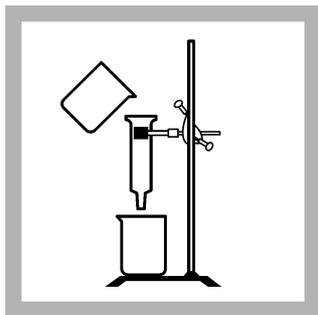
**10.** Slowly pour the prepared sample into the center of the extractor. Wait for the sample to flow through. The sample solution must flow slowly (2 drops per second) through the extractor. Keep the level of the sample solution just above the cotton plug.
