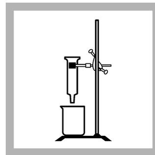
**12.** Put a clean, dry 150 mL beaker under the Extractor. Use a 25-mL plastic graduated cylinder to add 25-mL of pPb-3 Eluant Solution to the Extractor. Keep the level of the eluent solution just above the absorbent pad.
