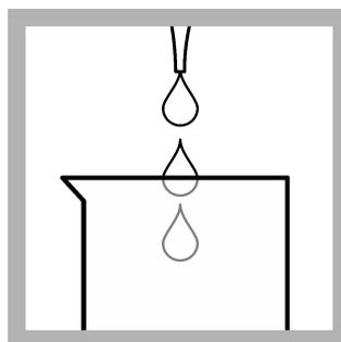
3. With a plastic 1 mL dropper, add 1.0 mL of pPb-1 Acid Preservative Solution to the sample.
