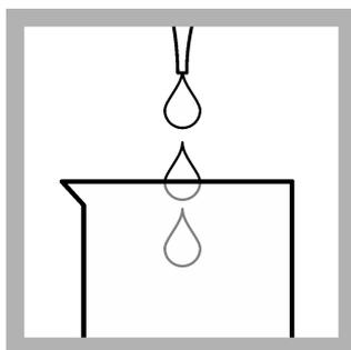
6. When the timer expires, use a second 1-mL plastic dropper to add 2.0 mL of pPb-2 Fixer Solution.
