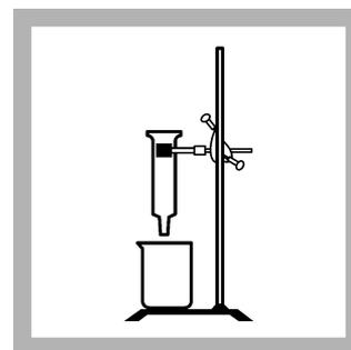
8. Install a new Fast Column Extractor in a ring stand with a clamp. Put a 150-mL plastic beaker under the extractor. The extractor is in the LeadTrak<sup>®</sup> Reagent Set. A new extractor is necessary for each test procedure.
