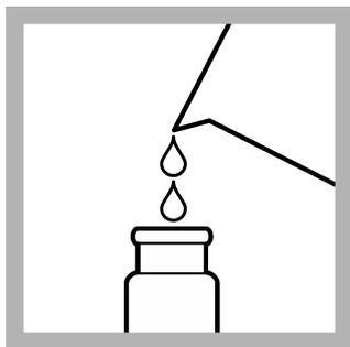
**18.** Pour 10 mL of the solution into a sample cell.
