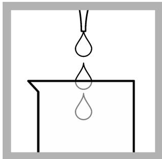
**14.** With a 1 mL plastic dropper, add 1.0 mL of pPb-4 Neutralizer Solution to the beaker.
