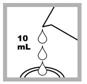
**21. Prepare the blank:** Fill a dry sample cell with 10 mL of chloroform. Put the stopper on the sample cell.
