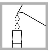
2. Fill a 250-mL graduated cylinder to the 250-mL mark with sample.
