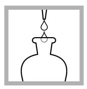
**16.** Add 5 more drops of 5.0 N Sodium Hydroxide Standard Solution. A pink color in the bottom (chloroform) layer in this step does not necessarily indicate that lead is in the sample. Only after potassium cyanide is added in the next step does a pink color confirm the presence of lead.
