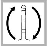
8. Put the stopper on the mixing cylinder. Invert the mixing cylinder several times to mix.
