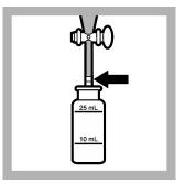
20. Prepare the sample: Put a cotton plug the size of a pea into the funnel delivery tube. Slowly drain the bottom (chloroform) layer into a dry 25-mL sample cell. Put the stopper on the sample cell. The lead-dithizone complex is stable for a minimum of 30 minutes if the sample cell is closed tightly and kept out of direct sunlight.
