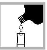
6. Prepare the DithiVer solution: Add 50 mL of chloroform to a 50-mL mixing cylinder.
