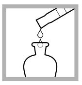
12. Add 5 mL of 5.0 N Sodium Hydroxide Solution to the funnel.
