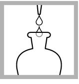
**15.** Add 3 drops of 5.0 N Sodium Hydroxide Standard Solution. Put the stopper on the funnel and shake to mix. Continue to add 3 drops and shake until the solution is orange. Large amounts of zinc cause the color change at the end point to be indistinct.
