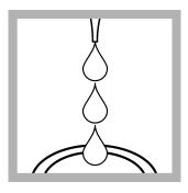
**6.** Add 12 drops of Alkaline Cyanide Reagent Solution to each cell.
