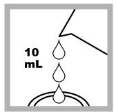
2. Prepare the blank: Fill the sample cell with 10 mL of deionized water. Digestion is necessary for total manganese determination.
