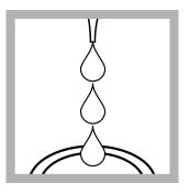
**8.** Add 12 drops of PAN Indicator Solution, 0.1% to each cell.
