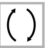
**6.** Put the stopper on the sample cell. Invert to mix. A violet color will show if manganese is present in the sample.
