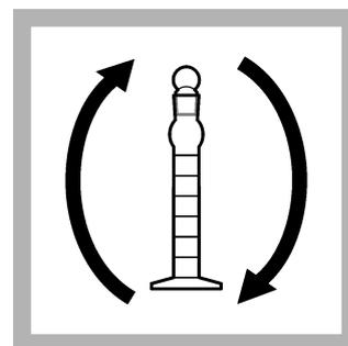
4. Put the stopper on the receiver. Invert to dissolve the reagent.
