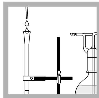
**8.** Pipet 2 mL of HgEx Reagent C into the Mercury Absorber Column.
