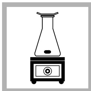
7. Use a watch glass as the flask cover. After the reagents dissolve, increase the temperature of the sample to 90 °C (194 °F). **Do not boil.**
