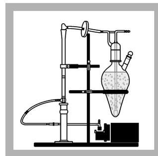
**12.** Use the quick disconnect to connect the vacuum pump to the Mercury Absorber Column again. Apply the vacuum to pull HgEx Reagent C through the Mercury Absorber Column packing and into the 10-mL receiver. Air bubbles should be produced at the gas dispersion tube in the Gas Washing Bottle. Complete the next two steps immediately.
