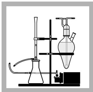
**6.** Use the quick disconnect to disconnect the vacuum pump when HgEx Reagent B starts to drip from the inner delivery tube on the Mercury Absorber Column (approximately 10 seconds after starting the vacuum). Make sure to not pull too much air through the Mercury Absorber Column, to prevent drying the packing.
