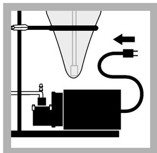
**17. Set the vacuum pump to off** when the volume in the Distilling Receiver is at the 10-mL mark. If necessary, adjust the volume in the Distilling Receiver a maximum of 10 mL with HgEx Reagent B.
