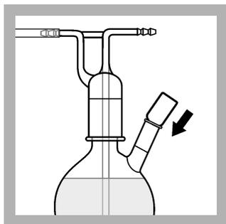
**10.** Shake an ampule of HgEx Reagent A to suspend undissolved reagent. Open the ampule and carefully pour the contents into the Gas Washing Bottle through the side neck.
