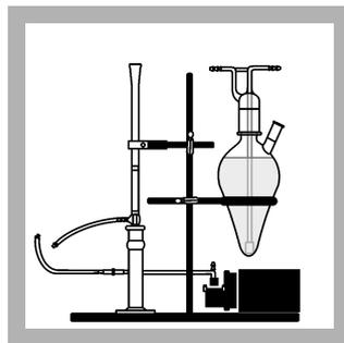
**7.** Remove the 100-mL Erlenmeyer flask from the Mercury Absorber Column. Replace it with the 10-mL Distilling Receiver.
