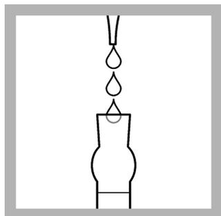
5. Add 8 drops of HgEx Reagent 5 to the Distilling Receiver.
