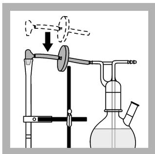
**9.** Use the glass elbow to connect the Mercury Absorber column to the Gas Washing Bottle.
