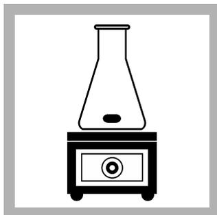
2. Put the flask on a magnetic stirring hot plate. Add a 50-mm magnetic stir bar to the sample. Set the stirrer power to on.
