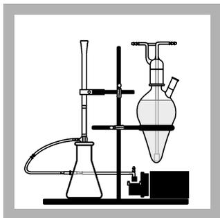
**5.** Apply a vacuum to the Mercury Absorber Column. Pull most of the HgEx Reagent B into the Erlenmeyer flask.
