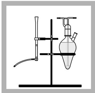
2. Set the Gas Washing Bottle in the support ring. Place the top on the Gas Washing Bottle. Wait until step 9 to connect the mercury absorber column to the Gas Washing Bottle.
