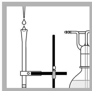
**19. Use a pipette to add 3 mL of HgEx Reagent B** into the Mercury Absorber Column without applying vacuum. This keeps the absorber packing wet between tests.
