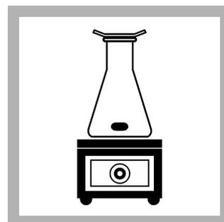
8. Continue to stir and keep the sample temperature at 90 °C for 2 hours. The solution must stay dark purple during the entire digestion. Some samples (e.g., seawater, industrial effluents or samples that are high in organic matter or chloride) require additional permanganate. It can be difficult to see a dark purple color if the sample contains black/brown manganese dioxide precipitate. Add more potassium permanganate if the solution is not dark purple.
