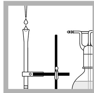
4. Pipet 8 mL of HgEx Reagent B into the Mercury Absorber column.
