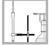
**19.** Use a pipette to add 3 mL of HgEx Reagent B into the Mercury Absorber Column without applying vacuum. This keeps the absorber packing wet between tests.
