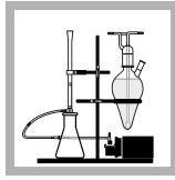
**5.** Apply a vacuum to the Mercury Absorber Column. Pull most of the HgEx Reagent B into the Erlenmeyer flask.
