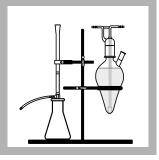
**18.** Remove the distilling Receiver from the Mercury Absorber Column. Connect the 100-mL Erlenmeyer flask to the column again.
