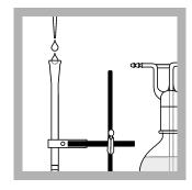
**16.** Pipet 8 mL of HgEx Reagent B into the Mercury Absorber Column to elute the captured mercury. Continue to apply the vacuum to pull the HgEx Reagent B into the Distilling Receiver.
