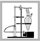
**12.** Use the quick disconnect to connect the vacuum pump to the Mercury Absorber Column again. Apply the vacuum to pull HgEx Reagent C through the Mercury Absorber Column packing and into the 10-mL receiver. Air bubbles should be produced at the gas dispersion tube in the Gas Washing Bottle. Complete the next two steps immediately.
