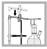
**9.** Use the glass elbow to connect the Mercury Absorber column to the Gas Washing Bottle.
