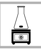
**2.** Put the flask on a magnetic stirring hot plate. Add a 50-mm magnetic stir bar to the sample. Set the stirrer power to on.
