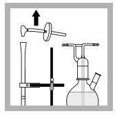
**15.** After the timer expires, remove the glass elbow from the top of the Mercury Absorber Column. Keep the vacuum pump power on.
