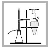
**3.** Connect the 100-mL Erlenmeyer flask to the mercury absorber column.
