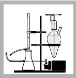
6. Use the quick disconnect to disconnect the vacuum pump when HgEx Reagent B starts to drip from the inner delivery tube on the Mercury Absorber Column (approximately 10 seconds after starting the vacuum). Make sure to not pull too much air through the Mercury Absorber Column, to prevent drying the packing.
