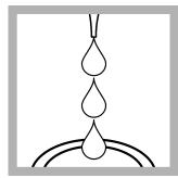
**6. Develop the sample:** Add 0.5 mL of Molybdenum 2 Reagent Solution to the prepared sample cell.
