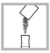
**3.** Add the contents of one Molybdenum 1 Reagent Powder Pillow to the mixing cylinder.
