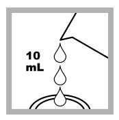
**5.** Fill a sample cell with 10 mL of the prepared sample.
