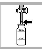
**14. Prepared sample:** When the timer expires, wait for the layers to separate. Put a cotton plug the size of a pea into the delivery tube of the funnel. Remove the stopper and drain the chloroform layer (the bottom layer) into a sample cell.
