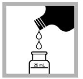
**17. Prepare the blank:** Fill a second sample cell with 10 mL of chloroform. Put the cap on the blank cell.
