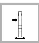
2. Measure 300 mL of the sample in a 500-mL graduated cylinder.
