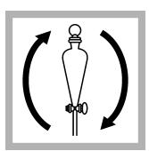
**11.** Put the stopper on the funnel. Carefully invert to mix. Make sure that the funnel tip is pointed up and away from people. Open the stopcock to release pressure.
