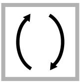
**16.** Put the cap on the sample cell. Invert to mix the extracts. The final volume is approximately 25 mL because of the slight solubility of chloroform in water.
