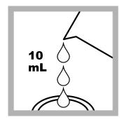
**12. Prepare the blank:** When the timer expires, fill a second sample cell with 10 mL of the original sample.
