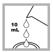
7. Prepare the sample: When the timer expires, carefully pour 10 mL of sample into a sample cell. Do not transfer cadmium particles to the sample cell.
