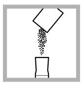
**3.** Add the contents of one NitraVer 6 Reagent Powder Pillow to the cylinder. Close the cylinder.
