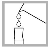
**2.** Fill the mixing cylinder with 15 mL of sample.
