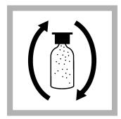
**5.** Use a stopper to close the Ampul tip. Invert the Ampul 48–52 times as the timer counts down.
