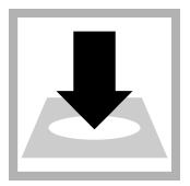
**11.** Within 2 minutes after the timer expires, insert the prepared sample AccuVac Ampul into the cell holder.
