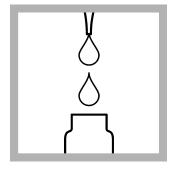
**1.** Use a pipet to add 1.0 mL of sample to the test vial.
