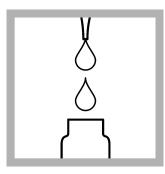
2. Use a pipet to add 1.0 mL of Solution A to the test vial
