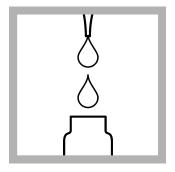
**1.** Use a pipet to add 0.2 mL of sample to the test vial.
