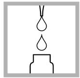
2. Prepare the sample: Fill a Test 'N Tube NitriVer 3 Nitrite vial with 5 mL of sample.
