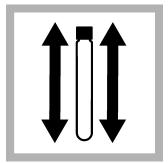
**3.** Put the cap on the vial. Shake to dissolve the powder. A pink color shows if nitrite-nitrogen is present in the sample .
