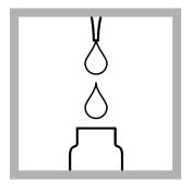
**5. Prepare the blank:** When the timer expires, fill and empty Test 'N Tube vial with 5 mL of sample.
