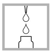
2. Use a pipet to add 2.0 mL of sample to the test vial. Immediately continue to the next step.
