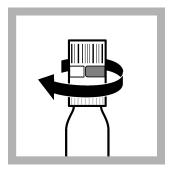
**3.** Turn the DosiCap Zip over so that the reagent side goes on the test vial. Tighten the cap on the vial.
