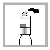
Carefully remove the lid from the DosiCap<sup>™</sup> Zip cap. Remove the cap from the test vial.
