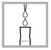
**8.** Use a pipet to add 1.0 mL of Nessler Reagent to each mixing cylinder.
