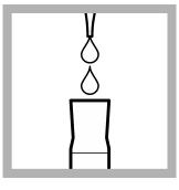
**6.** Add 3 drops of Polyvinyl Alcohol Dispersing Agent to each mixing cylinder.
