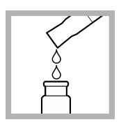
**15.** Pour 10 mL from the sample cylinder into a second sample cell.
