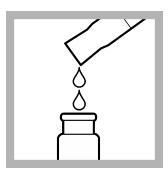
**11.** Pour 10 mL from the blank cylinder into a sample cell.
