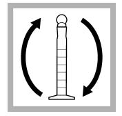
**5.** Put the stopper on the mixing cylinders. Invert the mixing cylinders several times to mix.
