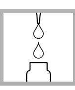
3. Prepare the sample: Add 0.1 mL of sample to one AmVer<sup>™</sup> Diluent Reagent Test 'N Tube for High Range Ammonia Nitrogen.
