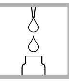
2. Prepare the blank: Add 0.1 mL of ammonia-free water to one AmVer<sup>™</sup> Diluent Reagent Test 'N Tube for High Range Ammonia Nitrogen.
