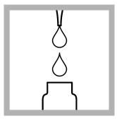
2. Use a pipet to add 5.0 mL mL of sample to the test vial. Immediately continue to the next step.
