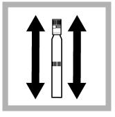
**4.** Shake the vial 2–3 times to dissolve the reagent in the cap. Look through the open end of the DosiCap to make sure that the reagent has dissolved.
