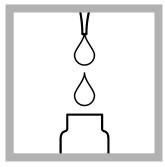
**2.** Use a pipet to add 0.5 mL of sample to the test vial. Immediately continue to the next step.
